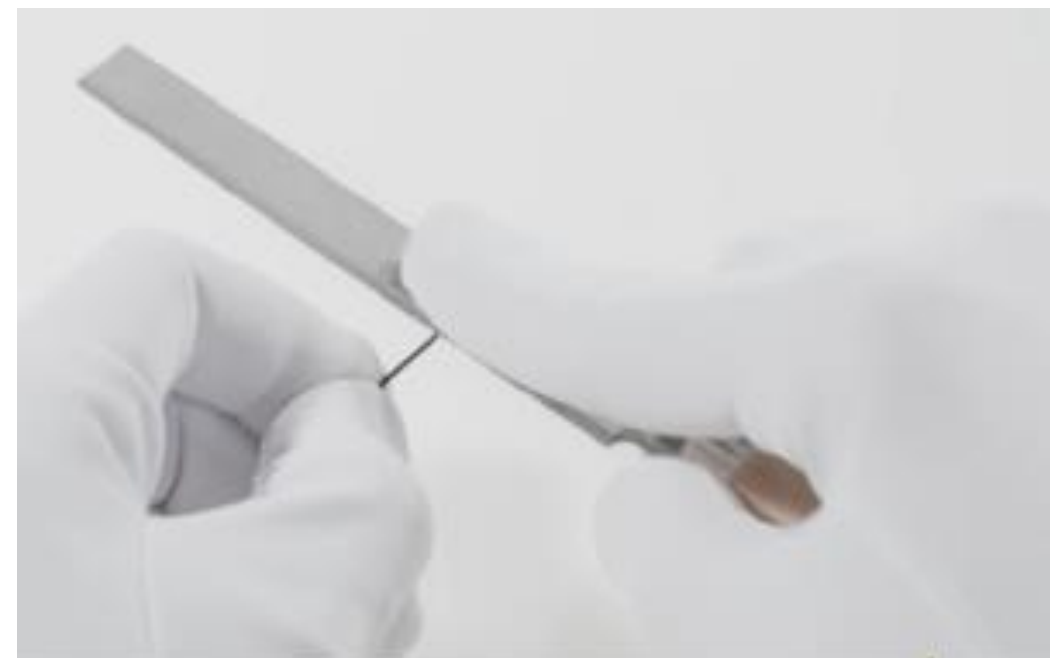
File down sharp edges and burrs
