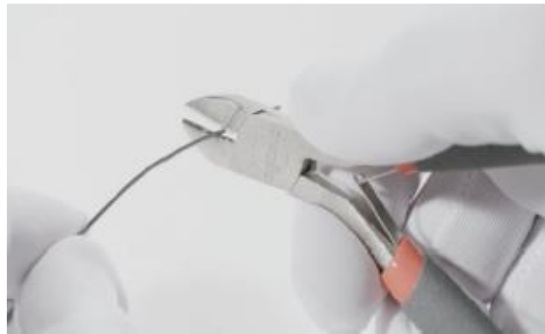
Remove temple cover and shorten stainless steel with diagonal cutter
